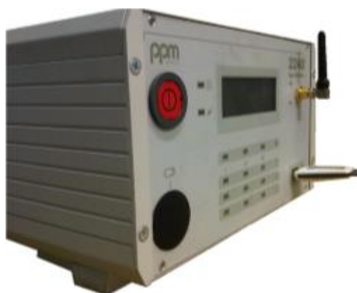
Picture 5. CertiPH3os phosphine monitor with GSM modem
