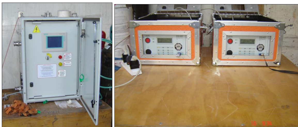
Picture 10 &11. HDS CF (left) used for continuous injection, controlled by CertiPH3os electronic phosphine monitors (right).
